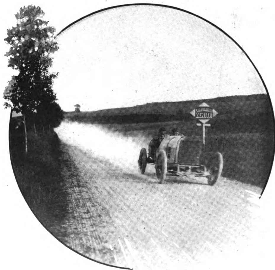
Fig. 1—Peugeot racer, Europe's fleetest speed production, which has swept the boards during the present season in long-distance road races, speed trials and hill-climbs. The machine, the development of racing engineers, is a light-weight, medium-powered creation, weighing under 2,000 pounds and with four cylinders 4.3-inch bore and 7.8-inch stroke, much smaller piston displacement than cars it has outdistanced. On road straightaways it has proven to be speedier than any cars entered in contests this year.
